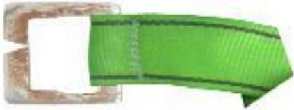
**Cracks on D-ring/ buckles**
