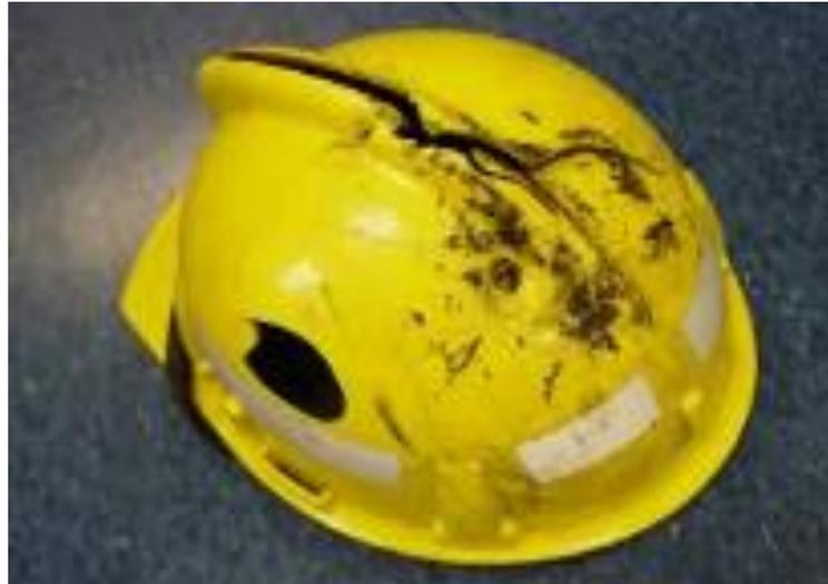
**look for cracks, dents, & cuts/gauges**
